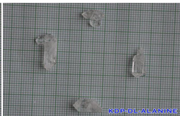
Figure: 2.3. DL-Alanine doped KDP Crystals
