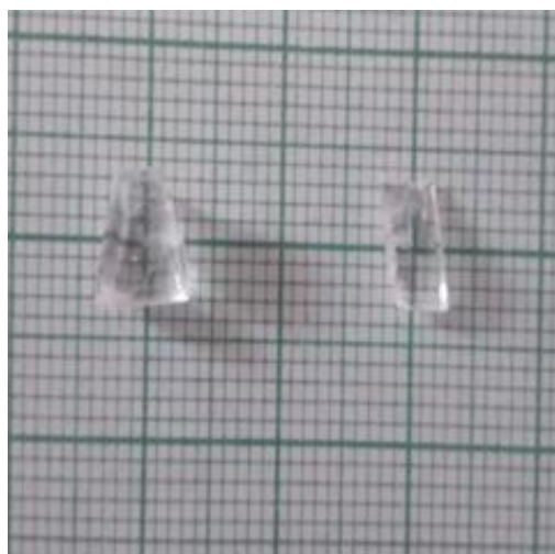
Figure 2. crystal of 0.2 % \text{Al}_2(\text{SO}_4)_3 doped TGS
