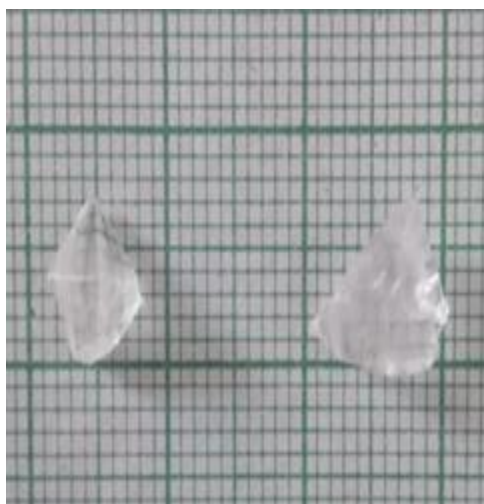
Figure 1. crystal of 1 % \text{Al}_2(\text{SO}_4)_3 doped TGS
