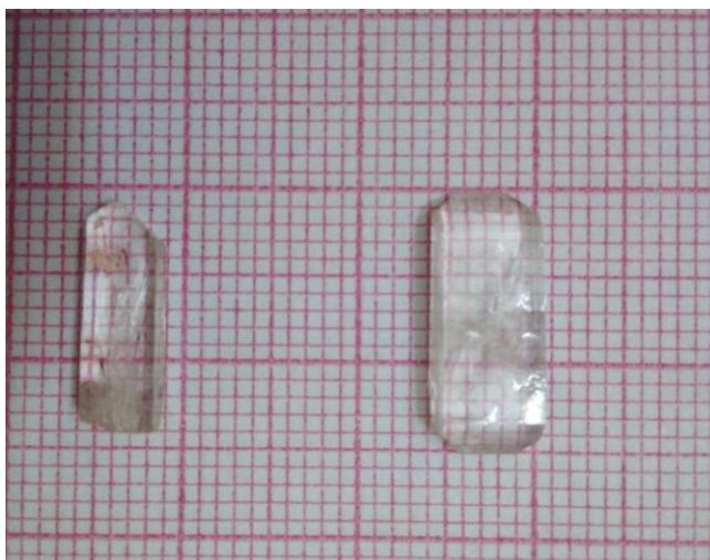
Figure 1. Grown crystal of KDPAP Single crystal
