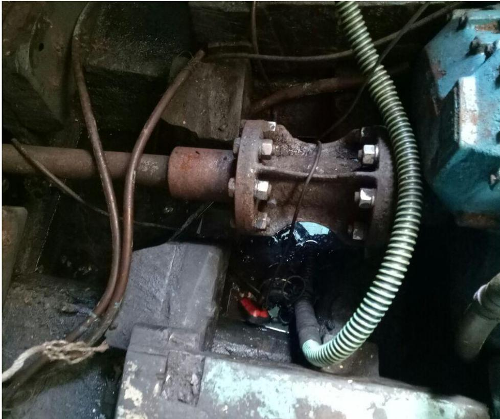
**Figure 3.** Submersible Pump at the Bottom of Bilge Tank
