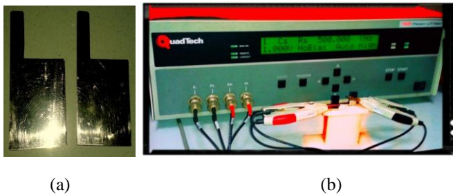
Fig. 2. Set up of capacitive sensor cell (a) electrodes (b) moisture sensor in working mode
