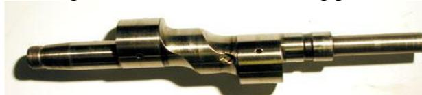
**Fig. 5** Eccentric shaft of Wankel Engine
