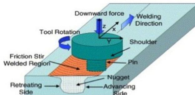
**Figure 1.** Schematic of the Friction Stir Welding process
