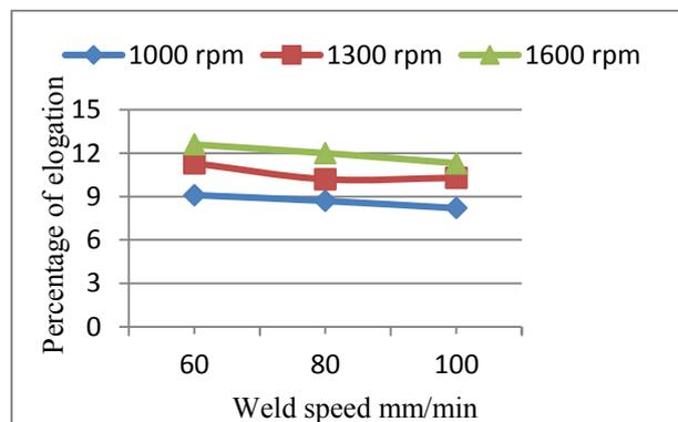
Figure 5. Effect of process parameters on percentage of elongation.
