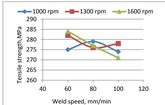
Figure 4. Effect of process parameters on tensile strength
