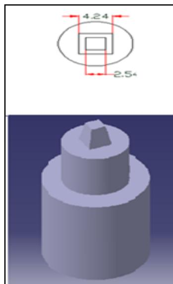
**Figure 2.** Geometry of a tapered square tool pin profile
