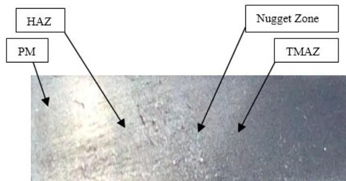
**Figure 7.** Macrograph of the welded sample
