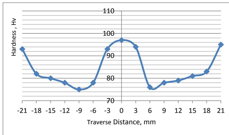
**Figure 9.** Hardness profile along the traverse direction
