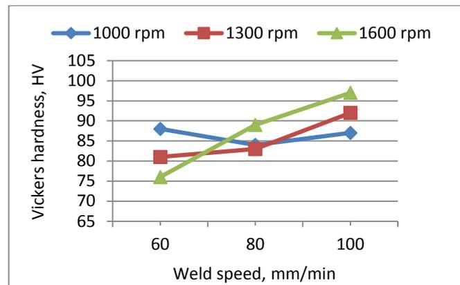
**Figure 6.** Effect of process parameters on the hardness
