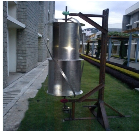
Fig. 4: Designed Model of the Windmill Fig. 5: Working Model of the Windmill
