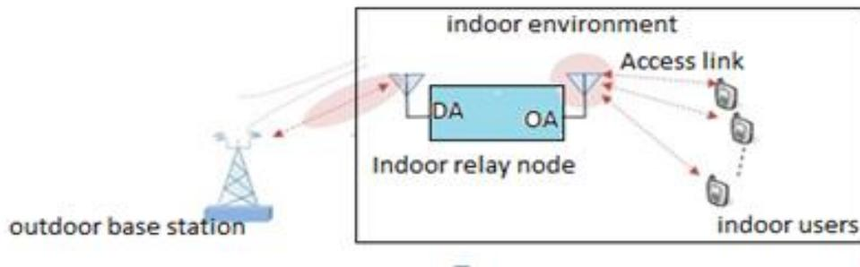
**Fig. 1** proposed an indoor relaying network
