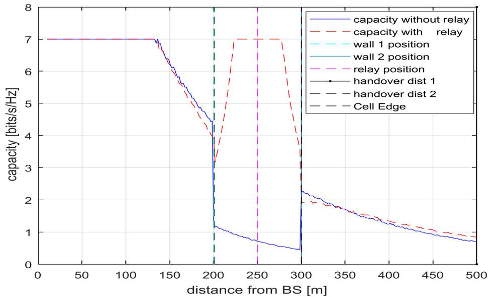
**Fig. 7** Performance of indoor capacity with relay over indoor capacity without relay
