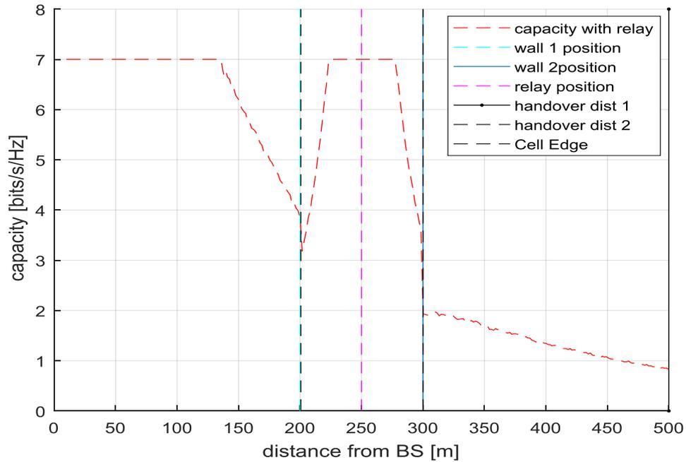
**Fig. 6** Indoor capacity with relay numerical values
