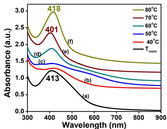
**Figure 2.** UV-vis spectra of chitosan/Ag nanocomposites using kumquat extract at various reaction temperatures: (a)  $T_{\text{room}}$ , (b) 40°C, (c) 50°C, (d) 60°C, (e) 70°C, and (f) 80°C, respectively.
