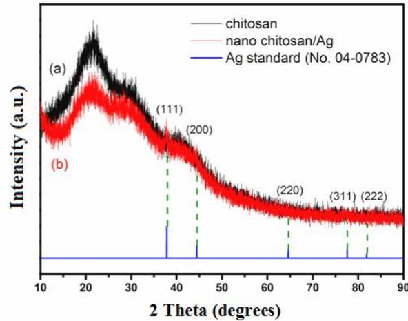
**Figure 6.** XRD patterns of (a) chitosan film and (b) chitosan/Ag nanocomposites film.
