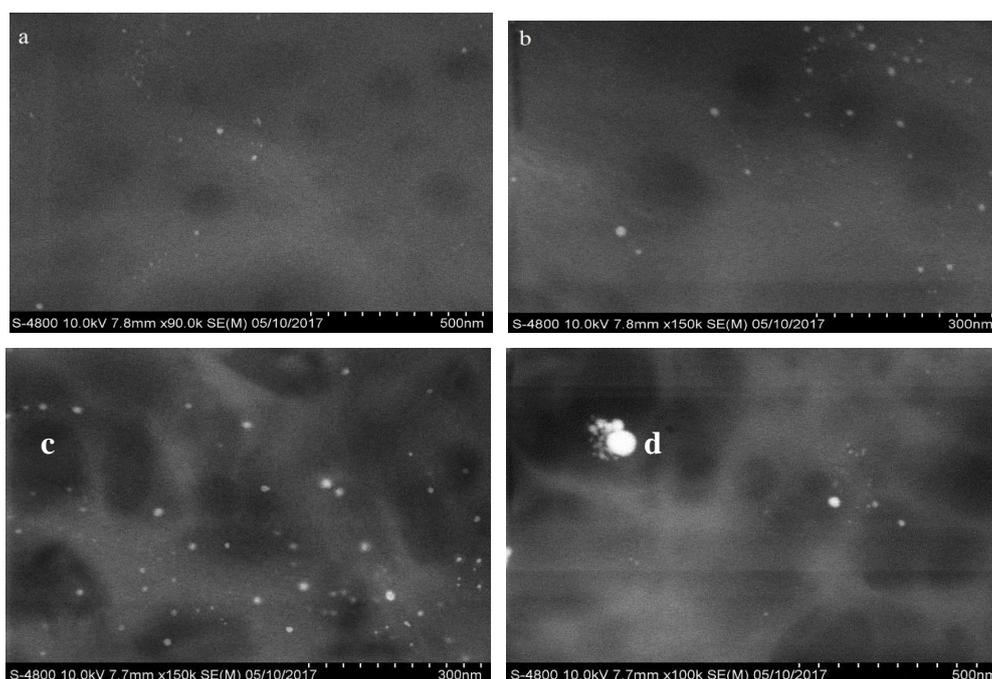
**Figure 4.** SEM images of chitosan/Ag nanocomposites films dried for 14 h in a vacuum oven at 70°C with different volumes of AgNO<sub>3</sub> solution (0.01 M): (a) 0.5 mL; (b) 1 mL; (c) 1.5 mL; (d) 2 mL, respectively.
