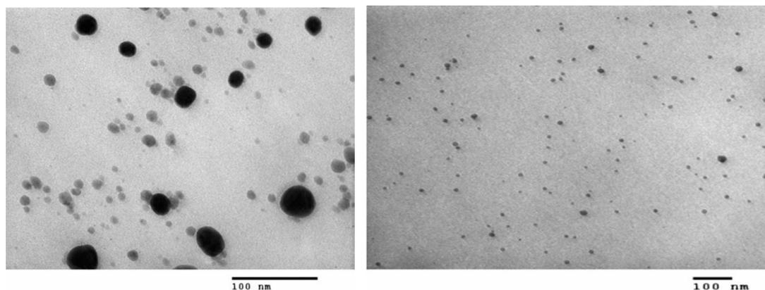
**Figure 3.** TEM images of chitosan/Ag nanocomposites (CTS/Ag NPs) using kumquat extract at 70 °C for 90 min.
