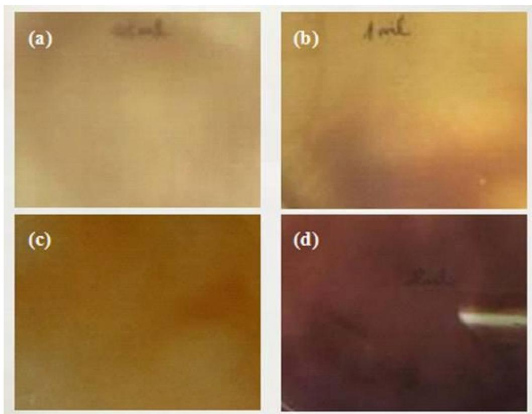
**Figure 1.** Photos of chitosan/silver nanocomposites (CTS/Ag NCPs) films dried in a vacuum oven for 14 h at 70°C with various volumes of AgNO<sub>3</sub> solution: (a) 0.5 mL; (b) 1 mL; (c) 1.5 mL; and (d) 2 mL, respectively.
