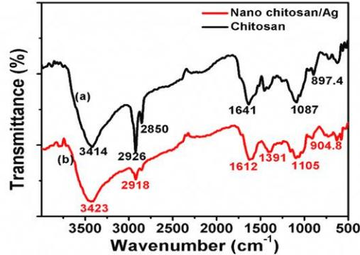
**Figure 5.** FTIR spectra of (a) chitosan film and (b) chitosan/Ag nanocomposites film.
