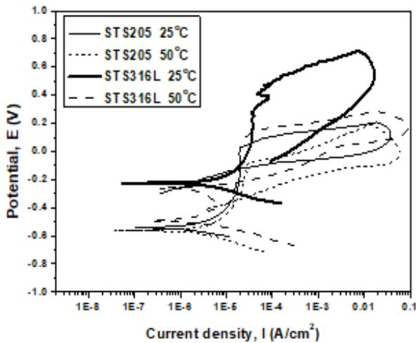
**Fig.3** Cyclic potentiodynamic polarization of specimens welds in NaCl solution
