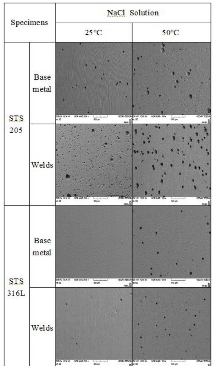
**Fig. 4** SEM micrographs of specimens base metal and welds after cyclic polarization test in NaCl solution.
