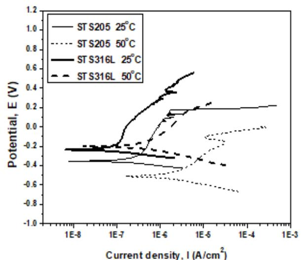
Fig.2 Potentiodynamic polarization curves of specimen welds in NaCl solution
