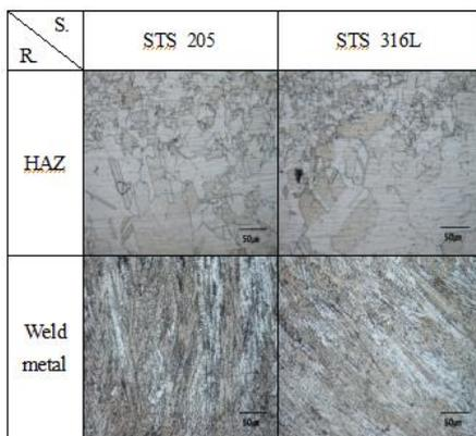
Fig.1 Optical microscope of GTAW specimens welds
