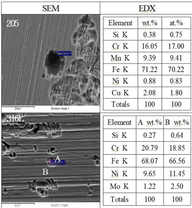
**Fig. 5** SEM/EDX results of pitting region from specimens welds in 50°C NaCl solution.
