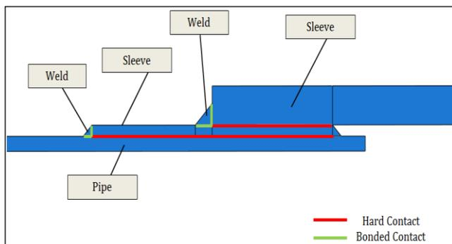
Figure 3: Contacts – Sleeve Assembly
