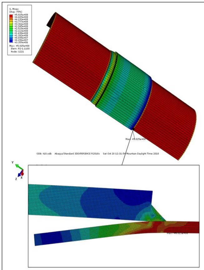
**Figure 5:** Von Mises Stress Plot – Operation (Pa)
