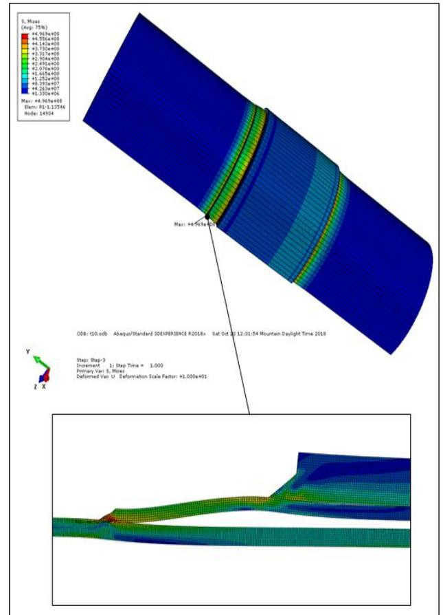
**Figure 6:** Von Mises Stress Plot - - Shutdown (Pa)
