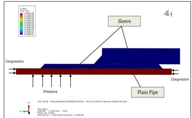
Figure 4: Initial States – Preloaded Plain Pipe (Von Mises: Pa)
