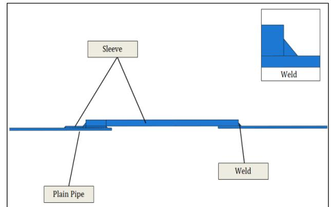
Figure 1: Model – Sleeve Assembly
