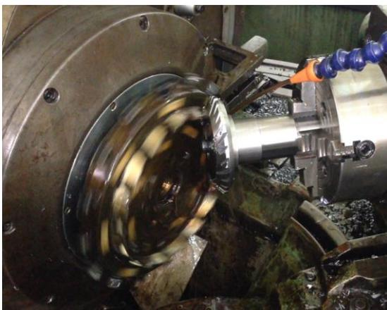
Figure 1. 525 specialized semi-automatic gear processing machine
