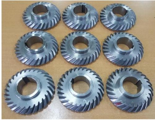
Figure 7. Post-processed gears
