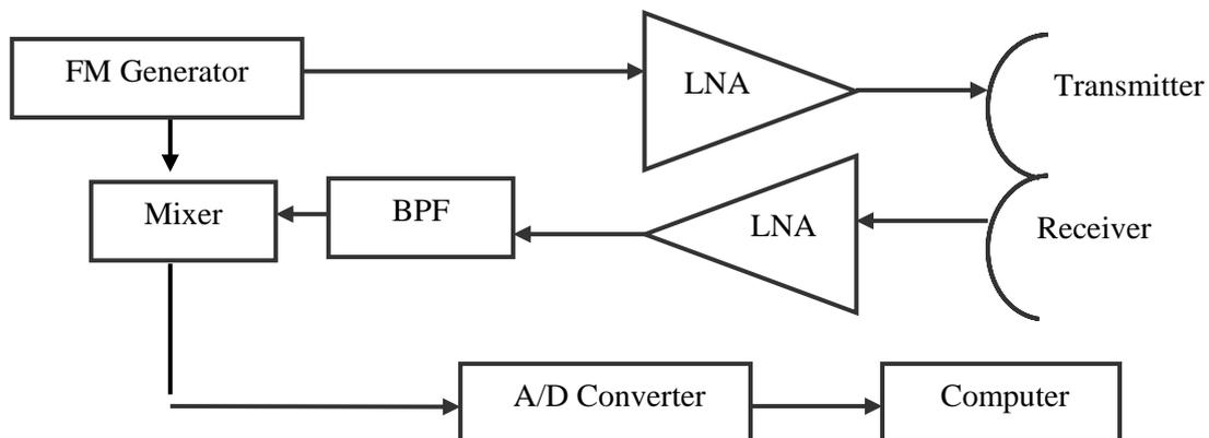
Figure 2. Block diagram of Final project design [3].
