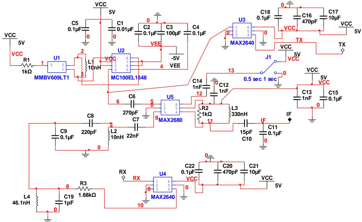
Figure 3. Final circuit of GPR.
