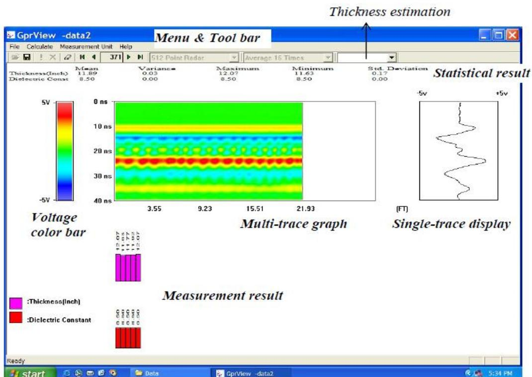
**Figure 10.** The interface for the GPR View software.
