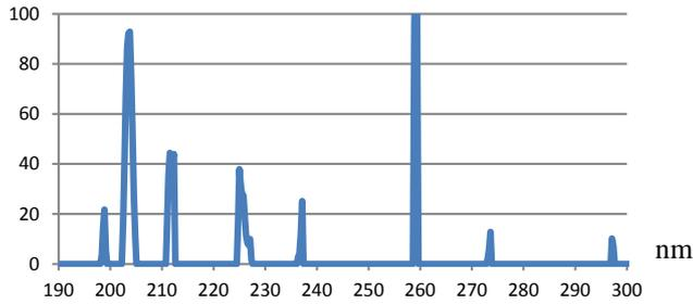
**Fig. 2.** The averaged difference emission spectrum from the area of the nickel cathode with a magnetic field.
