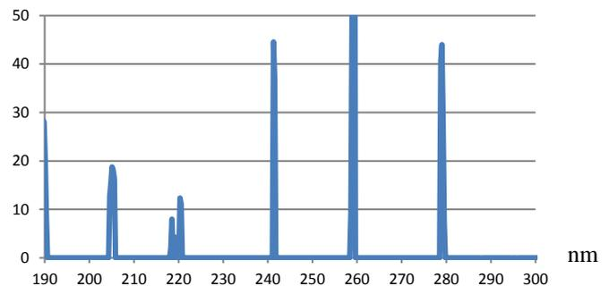
**Fig. 1.** The averaged difference emission spectrum from the nickel cathode area without a magnetic field.
