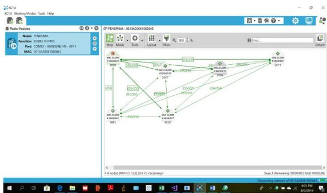
Figure 7. Result of connectivity testing between sensor nodes and coordinators using XCTU
