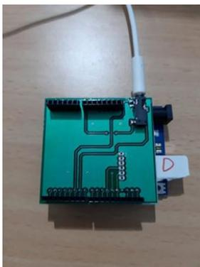
**Figure 4.** PCB a node sensor
