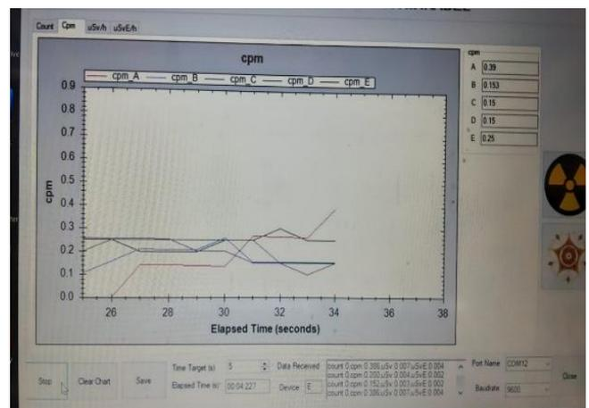
Figure 9. Background radiation is displayed in the GUI
