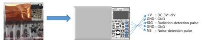
Figure 2. Radiation sensor and the interface specification
