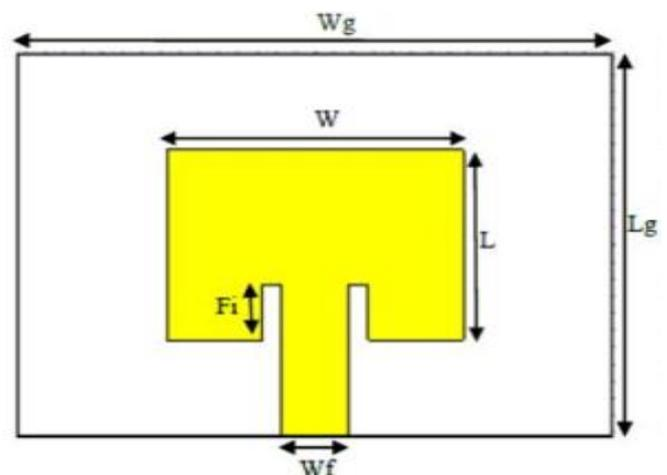
**Fig. 1:** Geometry of the proposed Microstrip patch antenna
