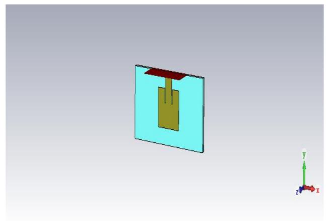
**Fig. 2:** Simulation environment of the proposed rectangular microstrip patch antenna
