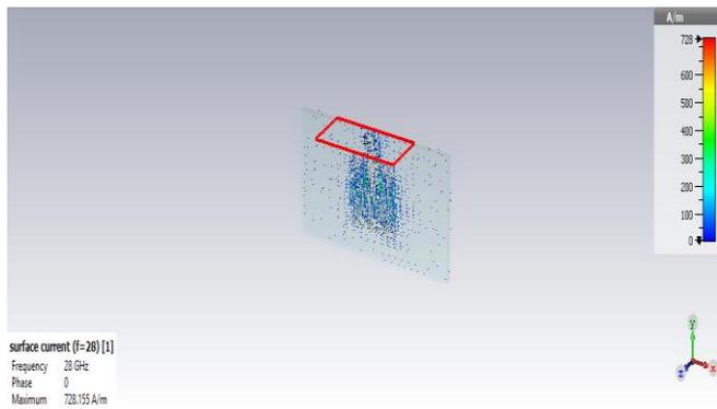
Fig. 7: Surface current distribution of the proposed antenna
