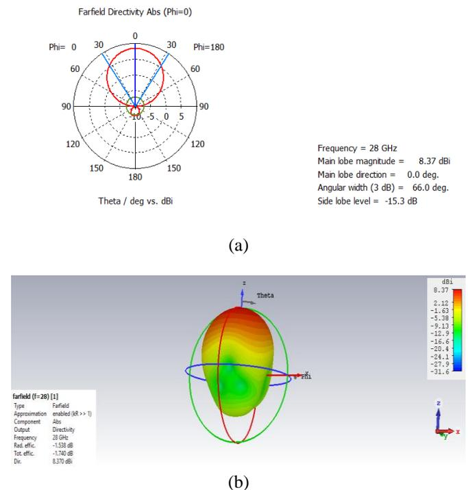
Fig. 6: (a) 2-D polar plot Radiation Patterns of the proposed prantenna at phi=0 (b) 3-D radiation pattern
