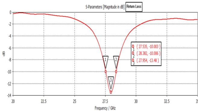
Fig. 3: Return Loss versus frequency of proposed antenna
