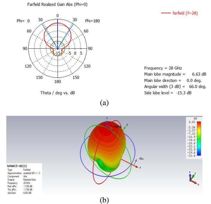
Fig. 5: (a) 2-D polar plot (b) 3-D Plot of the gain of the proposed antenna.
