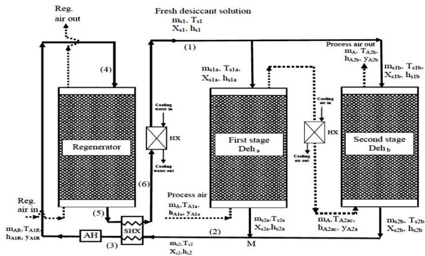
Fig.1a Schematic diagram for the proposed air dehumidification system A
