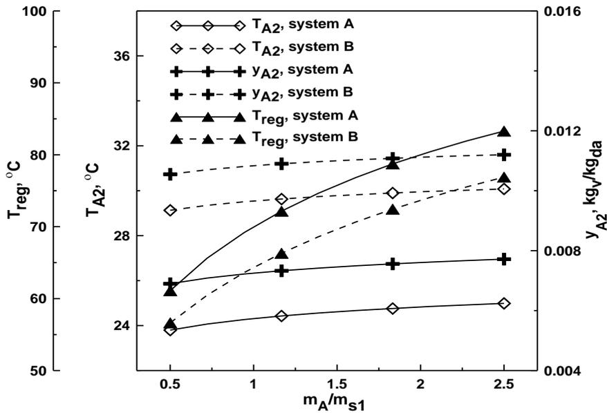
**Fig.6a** The effect of air to desiccant solution mass flow rate ratio ( $m_A/m_{s1}$ ) on  $T_{A2}$ ,  $y_{A2}$  and  $T_{reg}$ .
