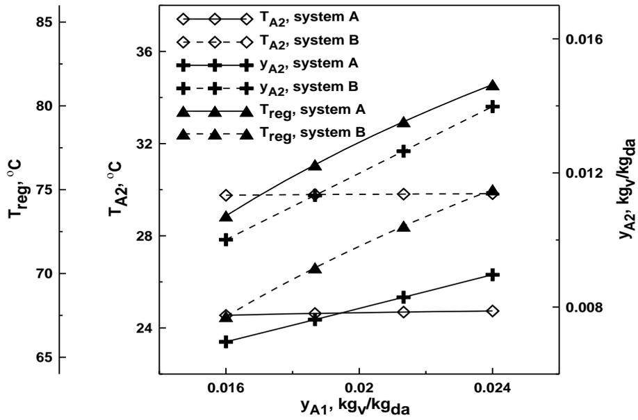
**Fig.2a** The effect of inlet air humidity ratio ( $y_{A1}$ ) on  $T_{A2}$ ,  $y_{A2}$  and  $T_{reg}$ .
