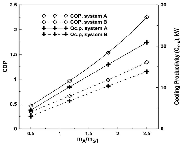
**Fig.6b** The effect of air to desiccant solution mass flow rate ratio ( $m_A/m_{s1}$ ) on COP and  $Q_{C,P}$ .
