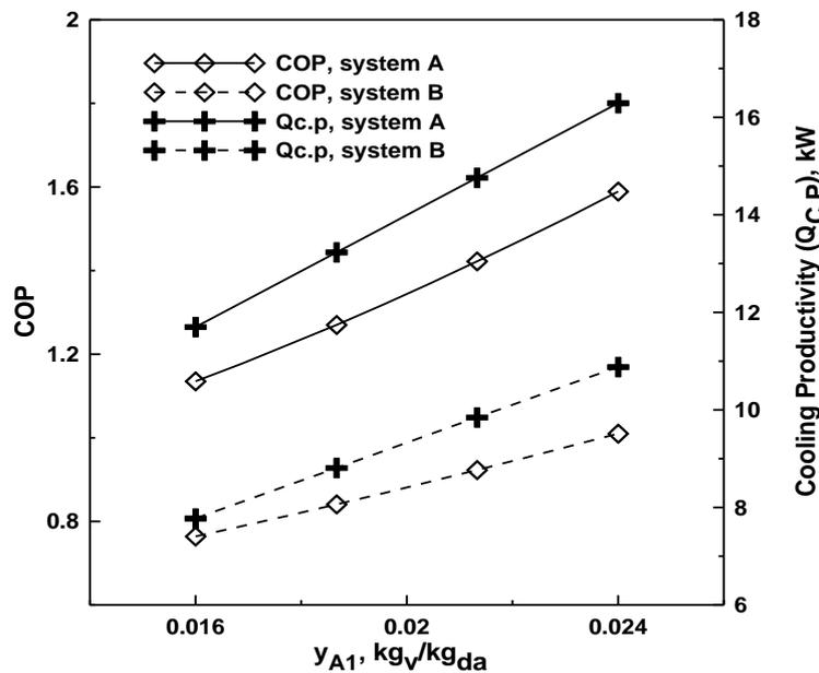
**Fig.2b** The effect of inlet air humidity ratio ( $y_{A1}$ ) on COP and  $Q_{c.p.}$ .
