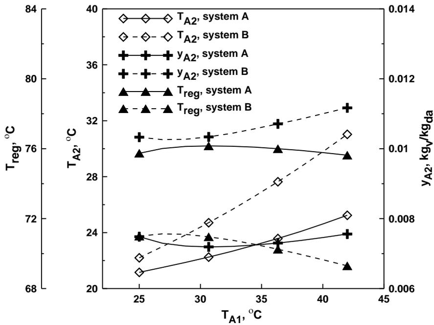
**Fig.3a** The effect of inlet air temperature ( $T_{A1}$ ) on  $T_{A2}$ ,  $y_{A2}$  and  $T_{reg}$ .
