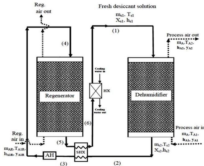
Fig.1b Schematic diagram for the proposed air dehumidification system B
