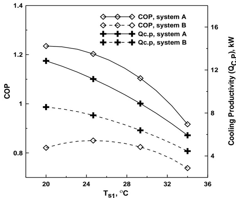
**Fig.5b** The effect of inlet desiccant solution temperature ( $T_{s1}$ ) on COP and  $Q_{C,P}$ .
