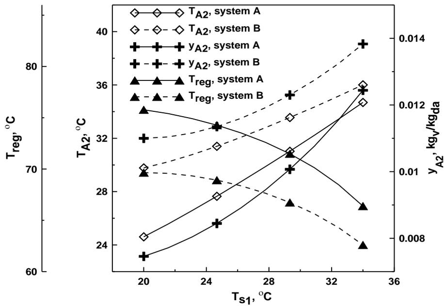
**Fig.5a** The effect of inlet desiccant solution temperature ( $T_{s1}$ ) on  $T_{A2}$ ,  $y_{A2}$  and  $T_{reg}$ .
