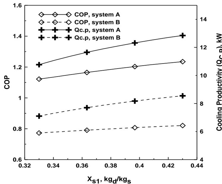
**Fig.4b** The effect of inlet desiccant solution concentration ( $X_{s1}$ ) on COP and  $Q_{C.P.}$ .
