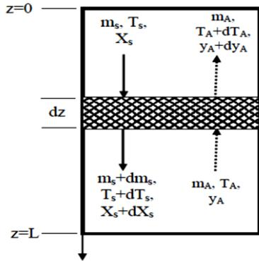
Fig.1c Elemental heat and mass transfer
