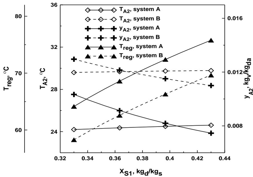
**Fig.4a** The effect of inlet desiccant solution concentration ( $X_{s1}$ ) on  $T_{A2}$ ,  $y_{A2}$  and  $T_{reg}$ .
