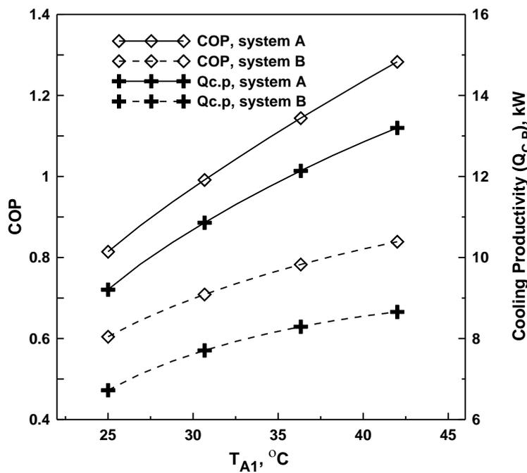
**Fig.3b** The effect of inlet air temperature ( $T_{A1}$ ) on COP and  $Q_{c.p.}$ .
