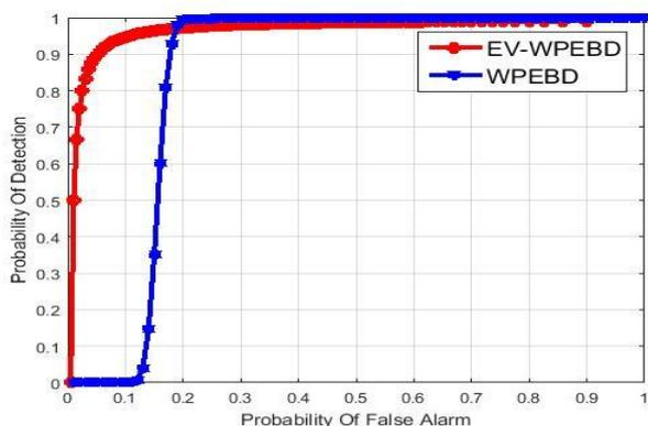
**Figure 5:** Comparison for Detection performance vs. false alarm probability for WPEBD and EV-WPEBD (SNR=-15 dB) and sample Size (N=18,000).
