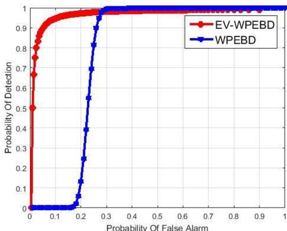
**Figure 6.** Comparison for Detection performance vs. false alarm probability for WPEBD and EV-WPEBD (SNR=-5 dB) and sample Size (N=18,000).
