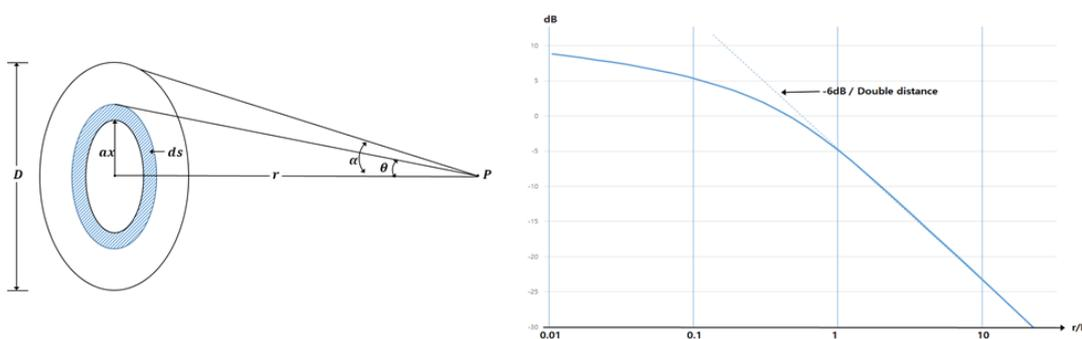
**Fig 4.** Distance attenuation of surface source [11]
