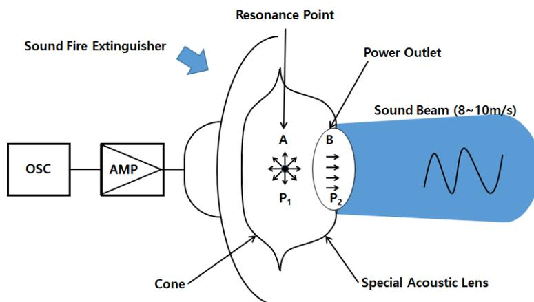
Fig 6. Sound Fire Extinguisher's sound beam formation
