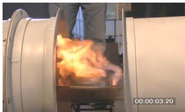
Fig 1. Sound Fire Extinguisher from DARPA[4]
