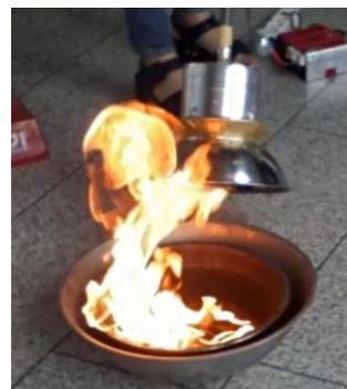
Fig 2. Sound Fire Extinguisher from SSERI
