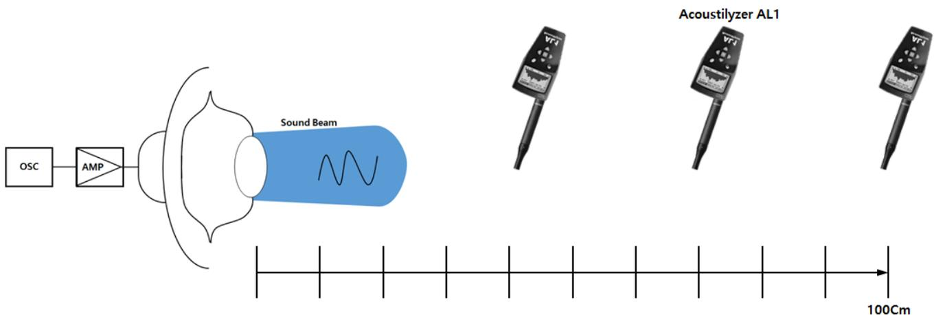
**Fig 8.** Measure sound level by distance
