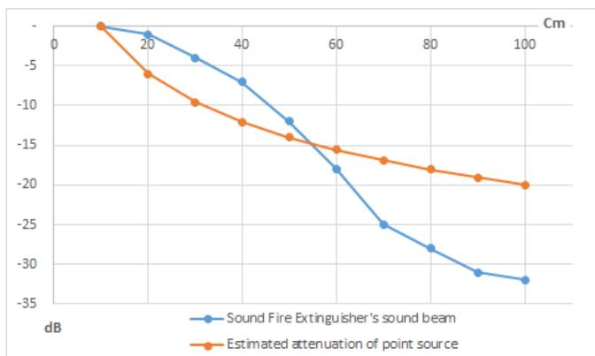
**Fig 9.** Comparison of attenuation by distance
