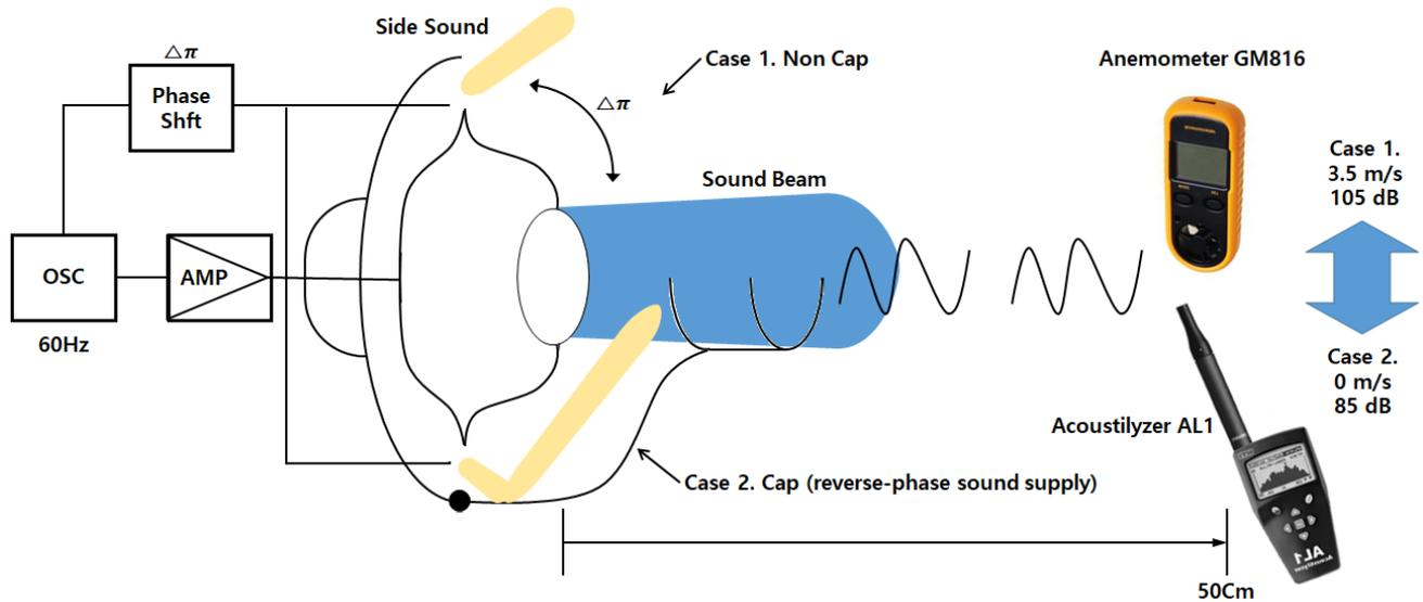
**Fig 7.** Comparison of wind velocity and sound level according to supply of reverse phase sound component
