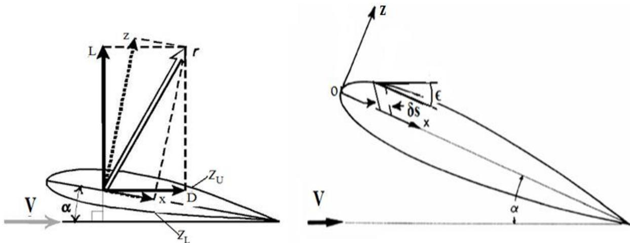
Figure 4. Normal pressure force on an element of the airfoil surface [15]
