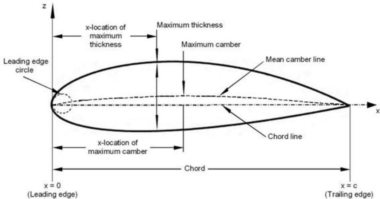
Figure 1. Airfoil-section geometry and its nomenclature [11]
