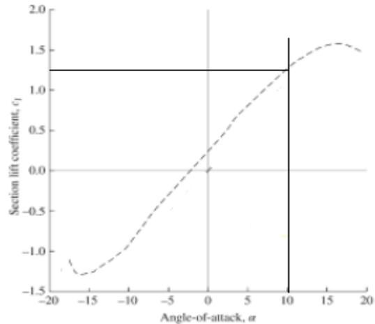
Figure 5. Lift coefficient vs. attack angle of NACA2412
