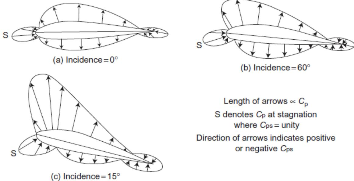
Figure 3. Typical pressure distributions on an airfoil section [15]
