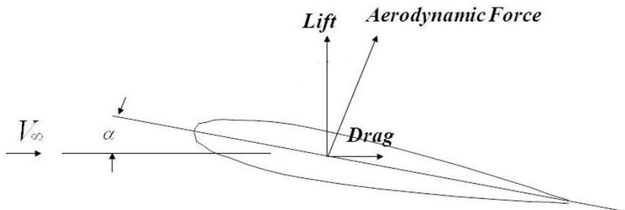
Figure 2. Aerodynamic forces [12, 14]
