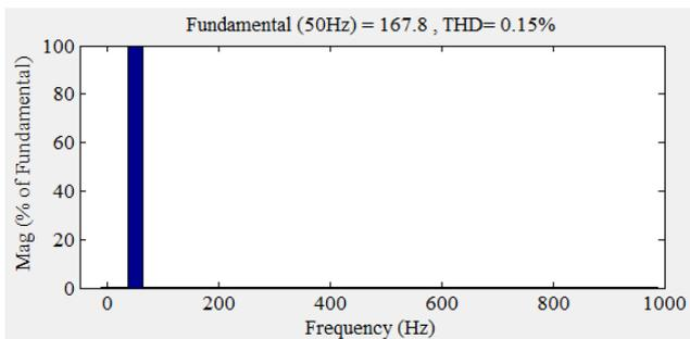
**Fig. 8.** THD of the fundamental current  $i_{LF}$  in steady-state with  $i_p$ - $i_q$  method
