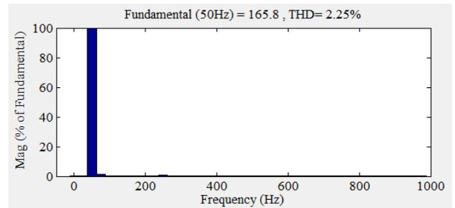
**Fig. 9.** THD of the supply current in steady-state with  $i_p$ - $i_q$  method
