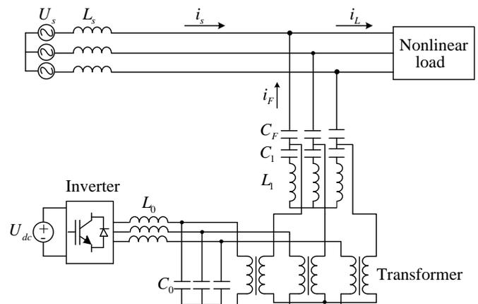
Fig. 5. Structure of a HAPF
