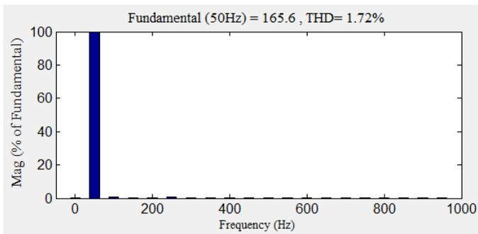
**Fig. 12.** THD of the supply current in steady-state with proposed method
