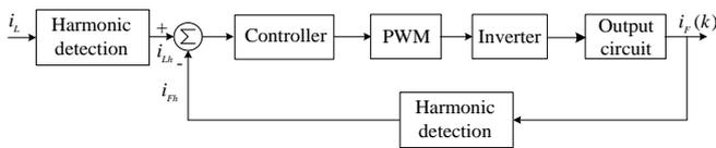
**Fig. 6.** Control block diagram for HAPF
