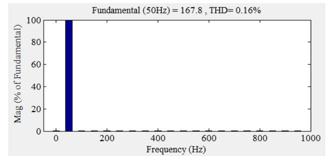
**Fig. 11.** THD of the fundamental current in steady-state with proposed method
