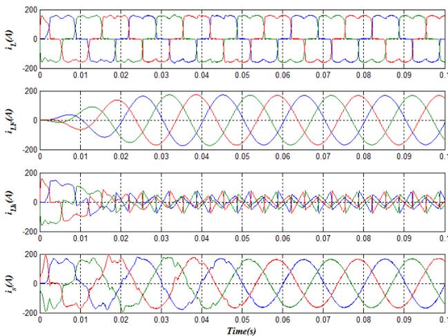
**Fig. 7.** Simulation results with the  $i_p$ - $i_q$  harmonic detection method
