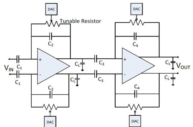
Figure 3: Generic architecture of neural recording channel.
