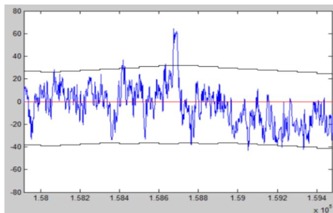
**Figure 1:** Measured noise in recording channel on PCB in AF5 chip.
