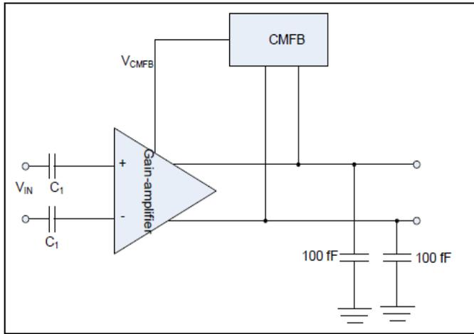
Figure 4: Second stage amplifier and compensating capacitor.
