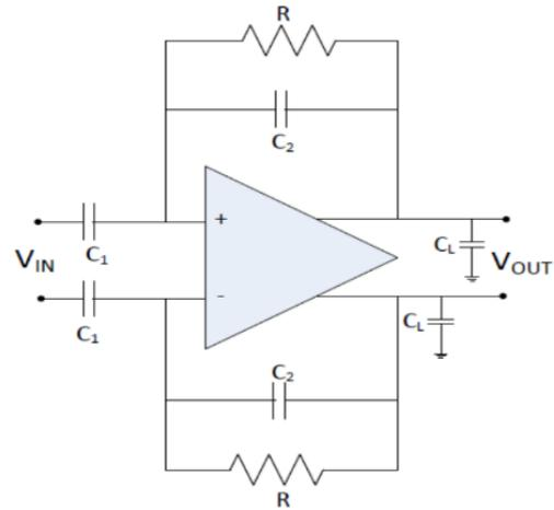
Figure 2: Band-pass filter for neural recording channel.
