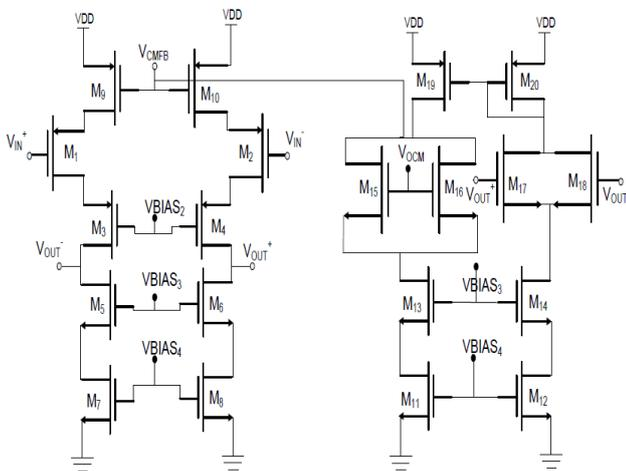
Figure 5: Schematic of LNA circuit and its CMFB circuit.
