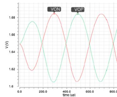
Transient simulation of the LNA.
