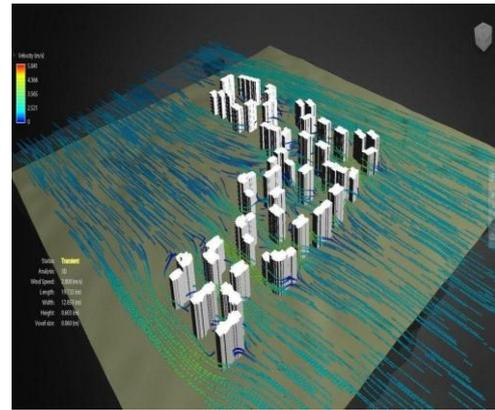
Fig. 3. Movement of easterly airflows at a speed  $V=2.0$  m/s
