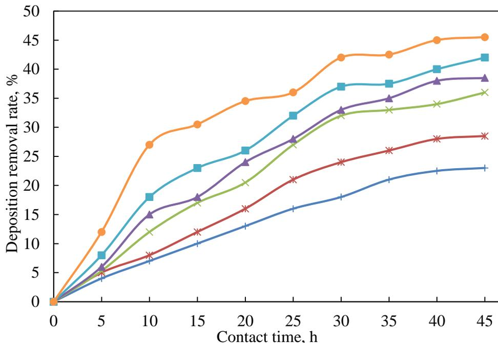
**Figure 1.** Kinetic curves of scale “washing off” at complexonate concentrations, where: —●— 20 mg/kg; —■— 15 mg/kg; —▲— 12 mg/kg; —×— 10 mg/kg; —\*— 8 mg/kg; —+— 4 mg/kg.
