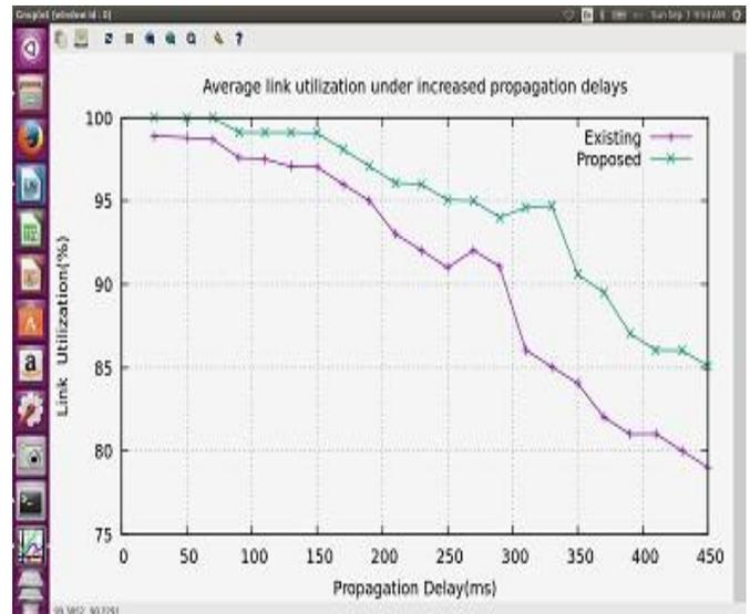
**Figure 3:** Average Link Utilization under Increased Propagation Delays
