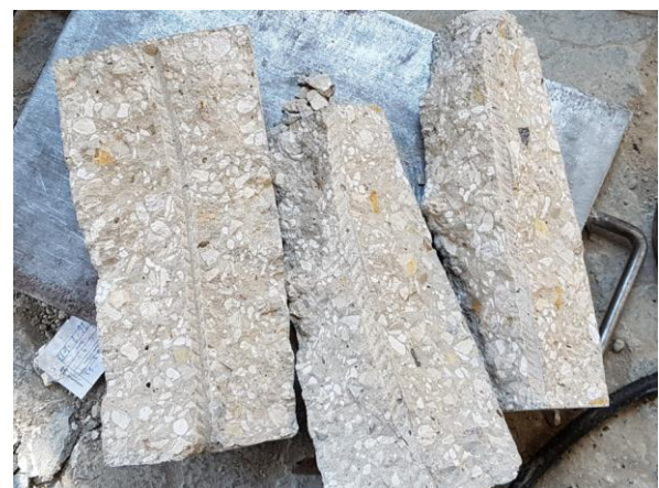
Figure 7. Used after segmentation deformed steel bar indentations
