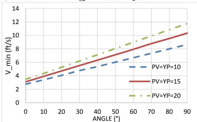
**Fig. 14.** Flow velocity vs. angle of inclination with variation of mud rheology from Rubi’s model.
