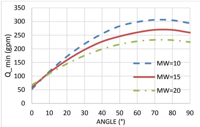
**Fig. 7.** Flow rate vs. angle of inclination with variation of MW from Larsen's model.
