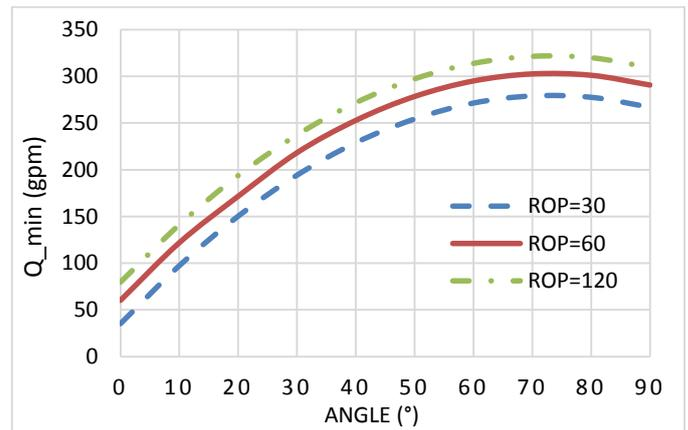
**Fig. 5.** Flow rate vs. angle of inclination with variation of ROP from Larsen's model.
