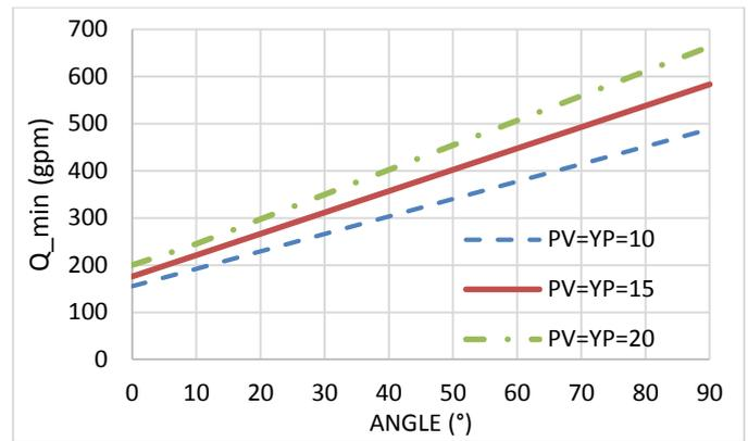
**Fig. 15.** Flow rate vs. angle of inclination with variation of mud rheology from Rubi’s model.
