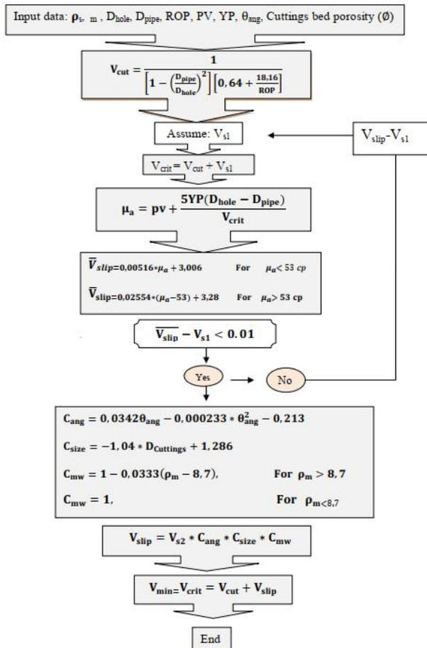
Fig. 2. Flowchart for calculating the velocity of drilling mud transport from Larsen's model [5, 6].
