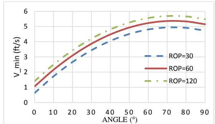
**Fig. 4.** Flow velocity vs. angle of inclination with variation of ROP from Larsen's model.
