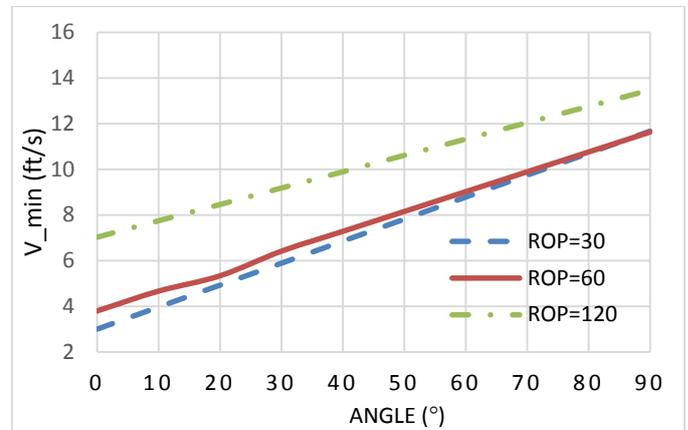
**Fig. 10.** Flow velocity vs. angle of inclination with variation of ROP from Rubi's model.
