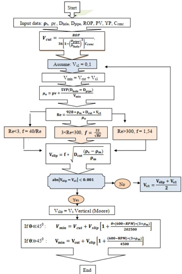
Fig. 3. Flowchart for calculating the velocity of drilling mud transport from Rubiandini's model [5, 6].
