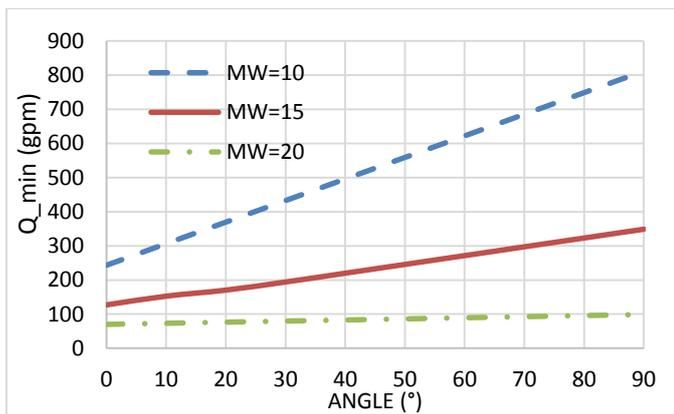
**Fig. 13.** Flow rate vs. angle of inclination with variation of MV from Rubi’s model.
