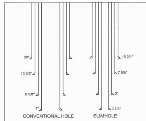
**Fig. 1.** Comparison of diameter of slimhole and conventional wells [2, 4].
