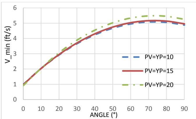
**Fig. 8.** Flow velocity vs. angle of inclination with variation of mud rheology from Larsen's model.
