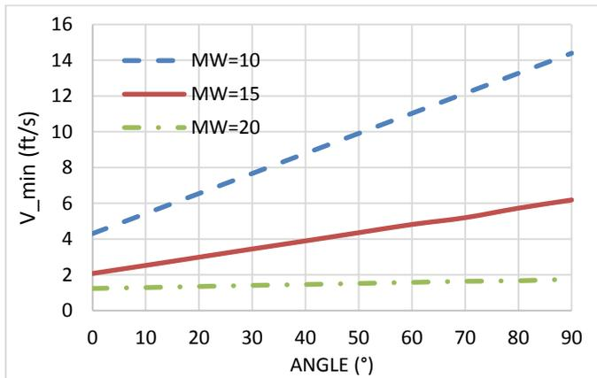
**Fig. 12.** Flow velocity vs. angle of inclination with variation of MV from Rubi’s model.
