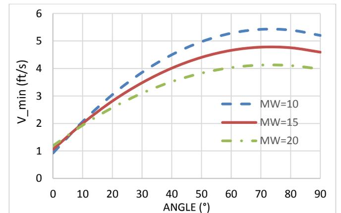
**Fig. 6.** Flow velocity vs. angle of inclination with variation of MW from Larsen's model.
