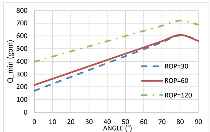
**Fig. 11.** Flow rate vs. angle of inclination with variation of ROP from Rubi's model.
