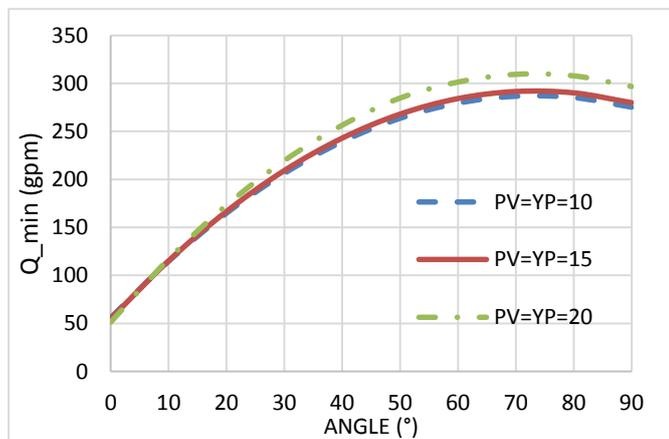
**Fig. 9.** Flow rate vs. angle of inclination with variation of mud rheology from Larsen's model.
