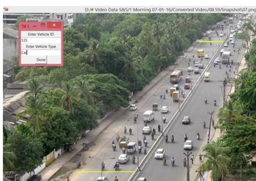
b) Screen Shot of GUI for Semi-Automated Vehicle Tracking
