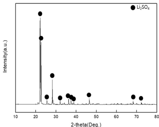
Fig. 1. XRD patterns of a raw specimen
