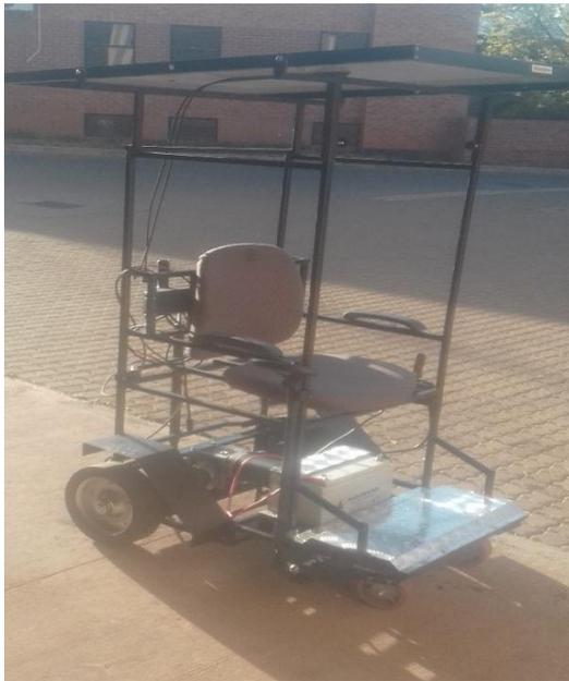
**Figure 3:** Solar-powered wheelchair
