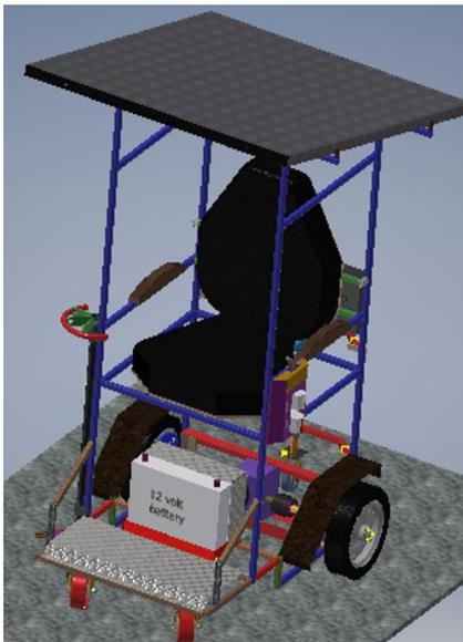
**Figure 1:** Design of solar-powered wheelchair
