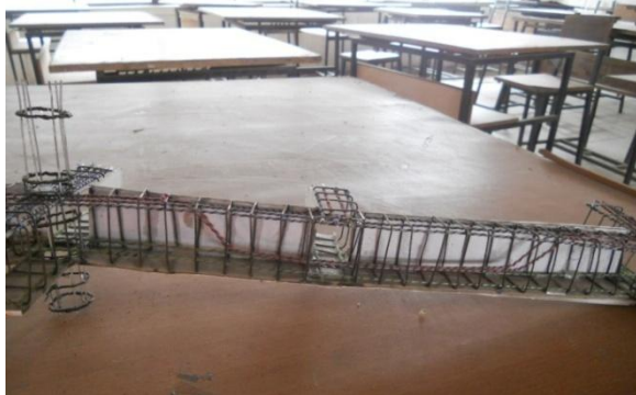
Image 6: Model of R.C.C. beam by students
