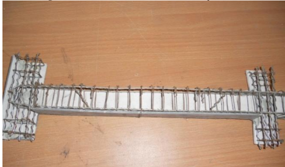
Image 7: Model of R.C.C. Beam by students
