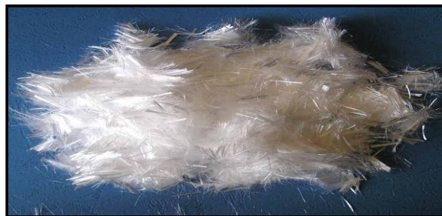
Fig-2 Polypropylene Fibers
