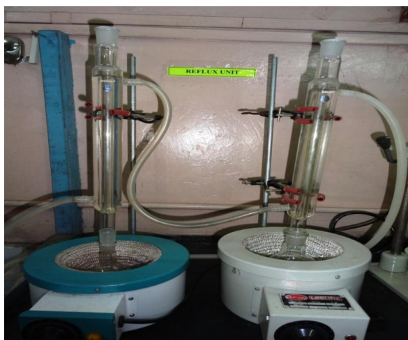
Figure 1: Actual photograph of the reflux method
