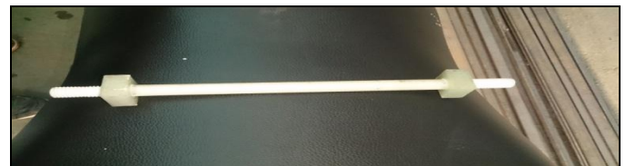
Photograph 1: Composite axle made by pultrusion process
