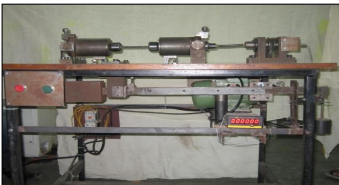
Photograph 5: Fatigue test set up
