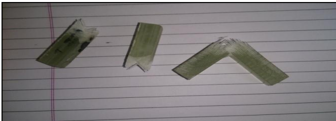
Photograph 4: Composite specimen after test
