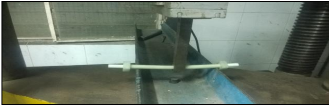
Photograph 3: Three point bending test set up
