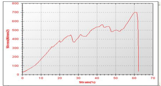
Fig 8: Stress-strain behavior of composite specimen
