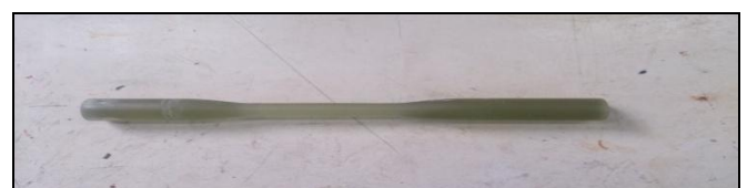
Photograph 2: Composite specimen for tensile test
