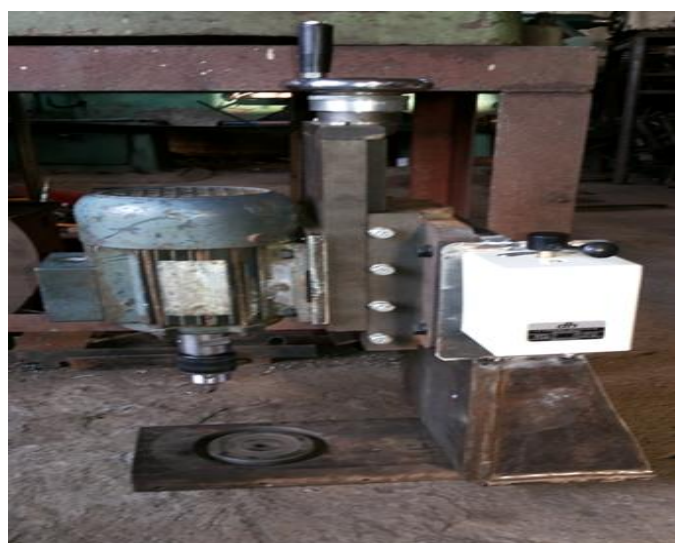
Figure 4: Setup With ON / OFF Switch
