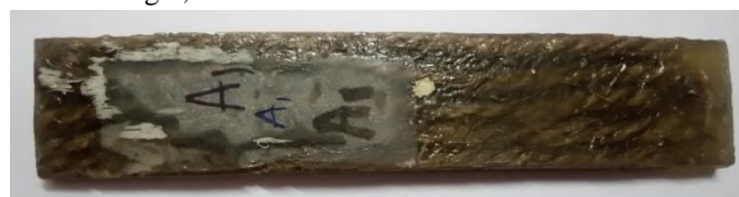
Fig 2.3 Flexural test specimen
