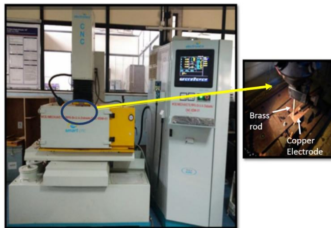
Figure 2 (b): Photograph of actual setup of R- \mu EDM process.
