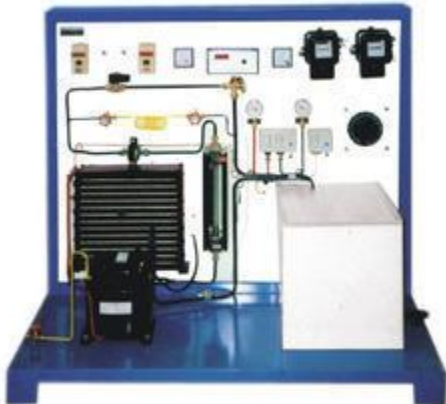
Figure 1: vapor Compression cycle.
