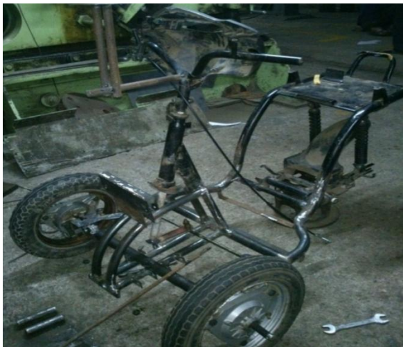
Image 4: Frame after Fabrication
