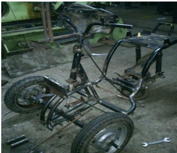
Image 4: Frame after Fabrication
