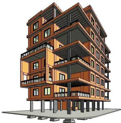
Figure 1: 3D model of the project prepared by the objects having definite material and geometric properties
