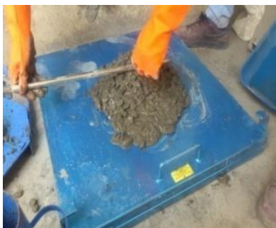
Fig.1 Flow table test
