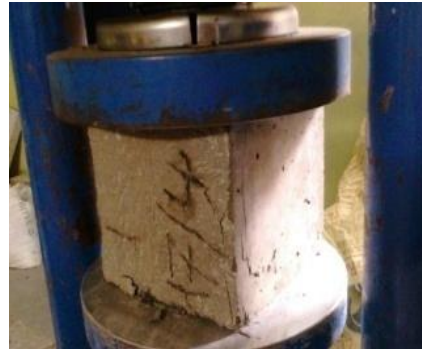
Fig.2 Compression test on cube
