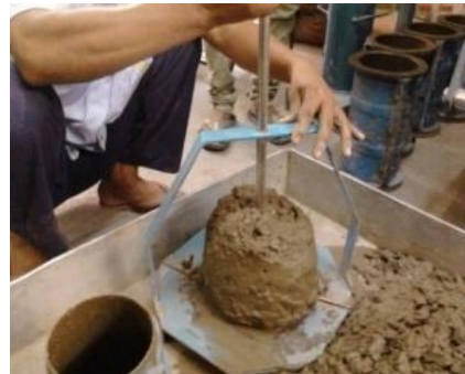
Fig.3 Slump cone test
