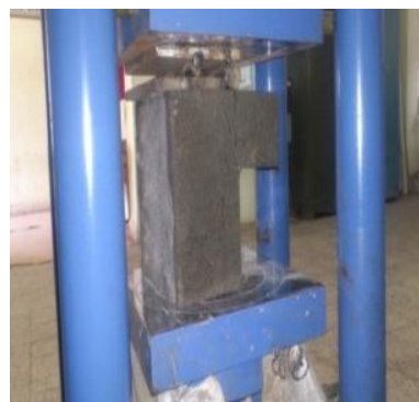
Fig4 Shear test on L shaped specimen
