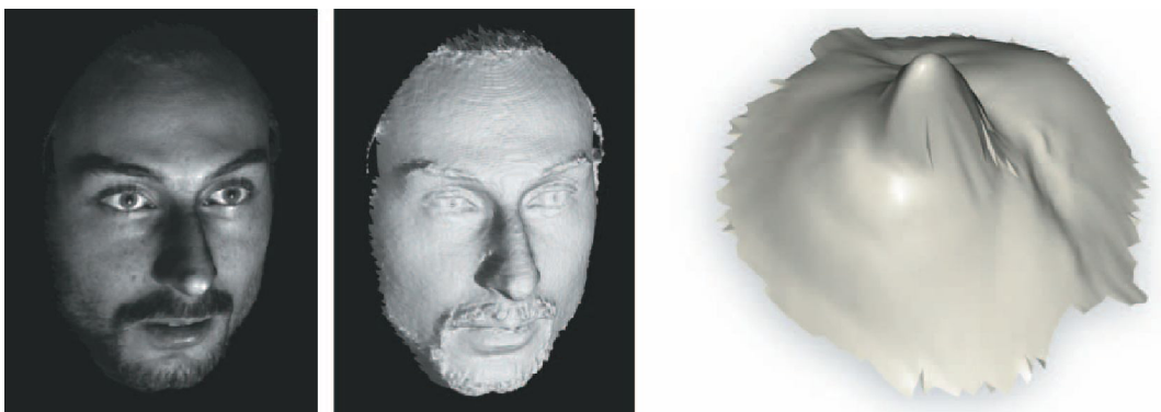
Figure 1: Three stages of facial recognition: (a) the range image and texture; (b) the pre-processed surface; (c) the canonical form.
