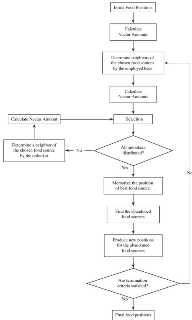
**Figure 4: Flowchart of the Artificial Bee Colony Algorithm.**
