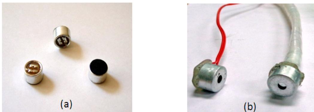
**Figure 2: (a) A snap shot of Condenser Microphones, (b) Condenser Microphone with wire attached for further connection to pulse sensor circuit.**
