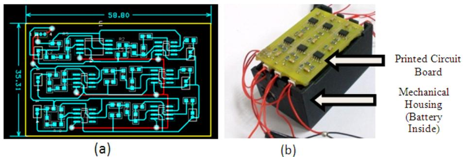
**Figure 4: (a) OrCAD PCB layout diagram for pulse sensor circuit (b) The pulse sensor circuit with battery connected inside the mechanical housing**
