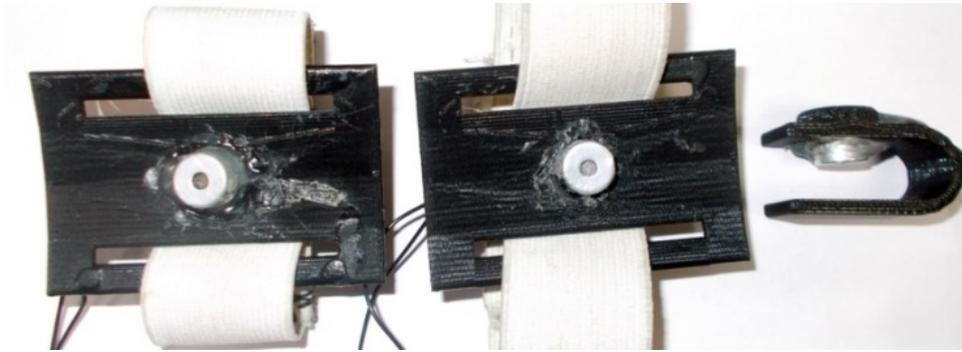
**Figure 3: Condenser Microphone placed in plastic housing rectangular shaped for Brachial, Radial artery region and u-shaped for Digital artery region**
