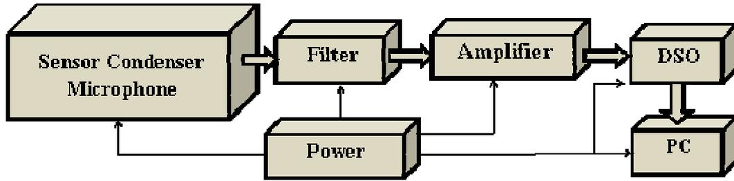
**Figure 1: Block diagram of the Pulse Sensor Circuit**
