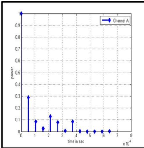
Multipath delay profile of channel A
