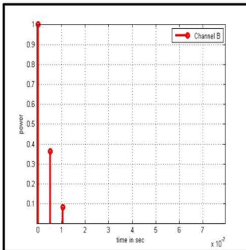
Multipath delay profile of channel B
