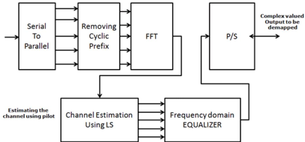
**Fig.1. Block diagram of IEEE 802.11a receiver**
