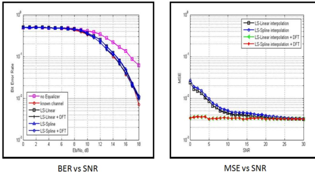
Fig-7: Performance in Channel C using different Channel Estimators
