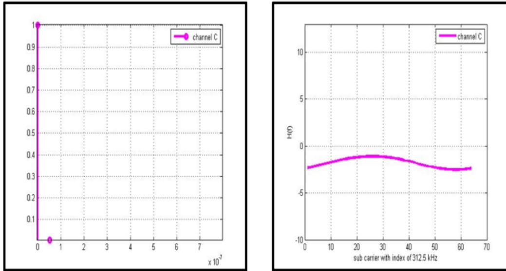
**Fig-4: PDP and frequency response of channel C**
