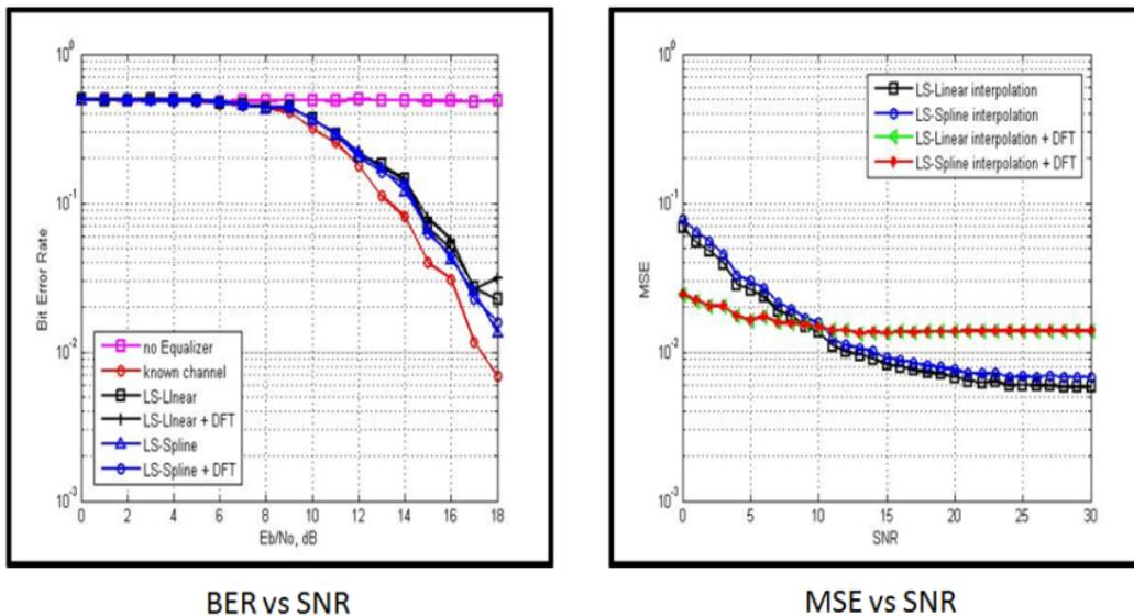
**Fig-5: Performance in Channel A using different Channel Estimators**
