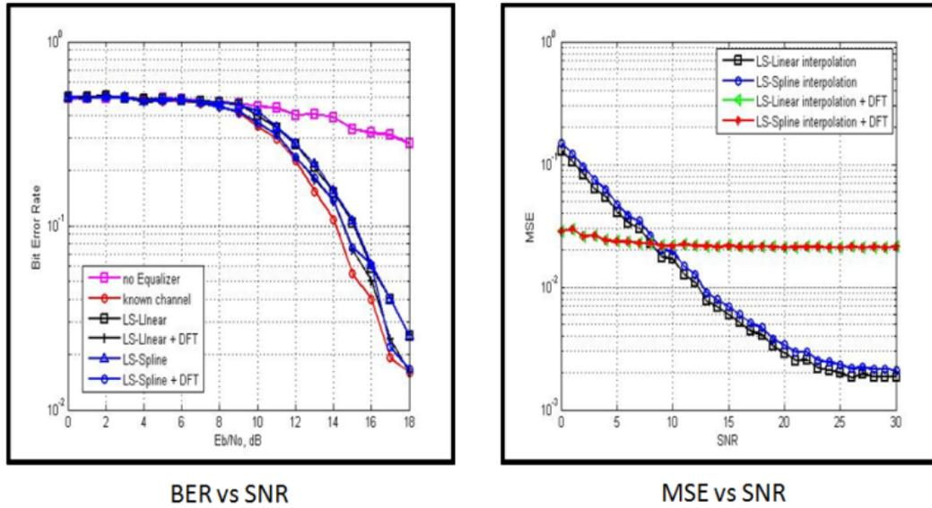
Fig-6: Performance in Channel B using different Channel Estimators
