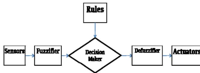
Fig. 1: Proposed interior structure of a single agent.
