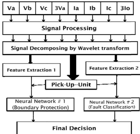
**Fig. 5:** Transmission line boundary protection scheme [13]
