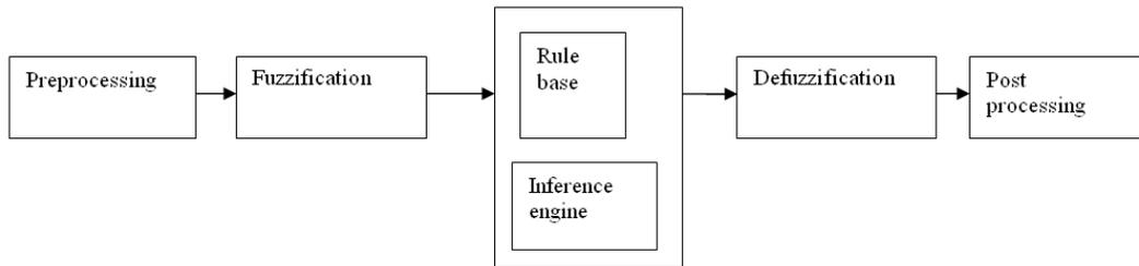
**Figure1:** Arrangement of fuzzy logic controller [1]
