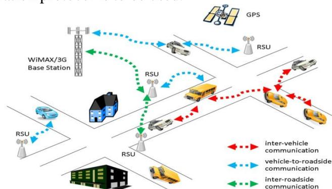
**Fig 1:** Block Diagram of VANET
